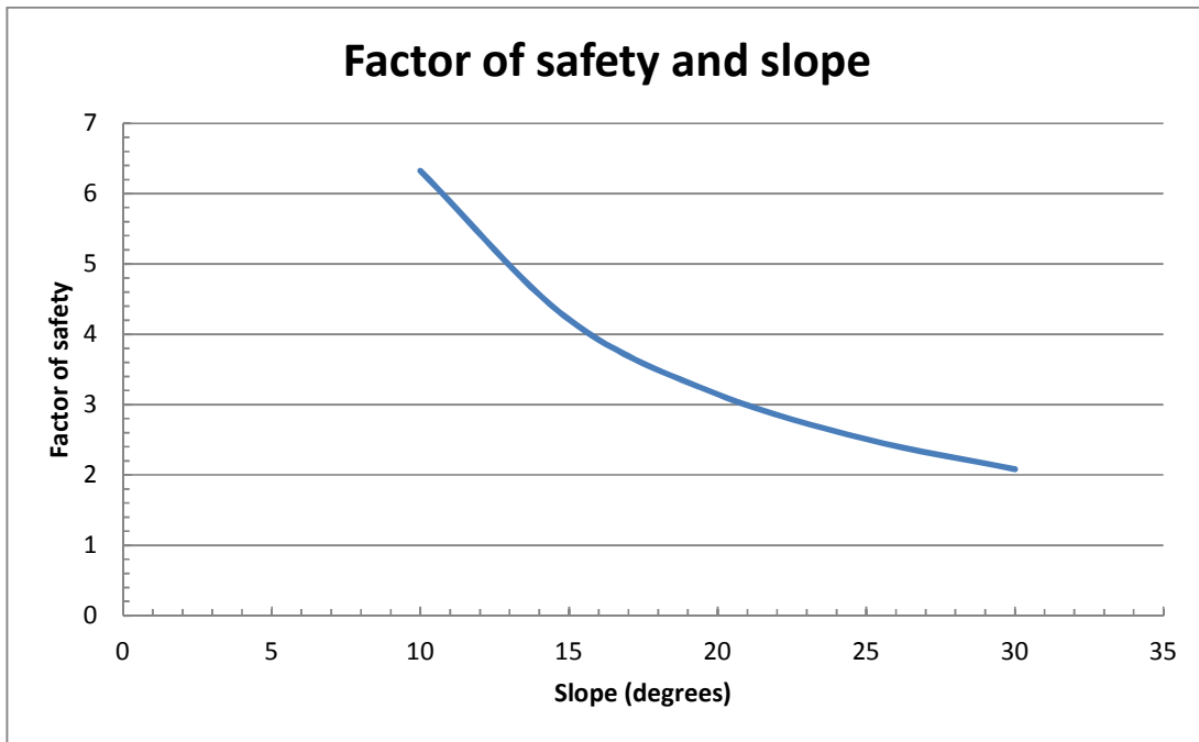
Fig. 1. Relationship between factor of safety and slope angle
