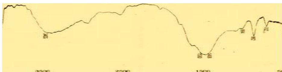
Fig. 7. Cd (II) loaded FTIR spectra of A. ferussacianus shell
