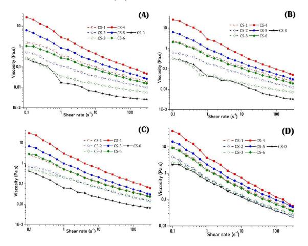
Fig. 4. Viscosity of control and calcium-enriched soymilk as function of shear rate at different storage time; (A) fresh, (B) 7 days, (C) 14 days and (D) 21 days
