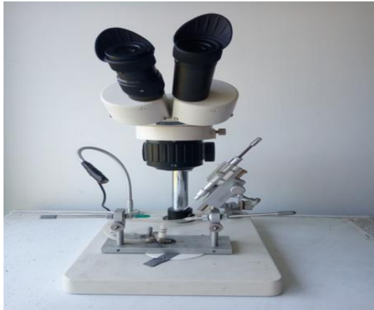
Fig. 3. Schely's instrumental insemination device
