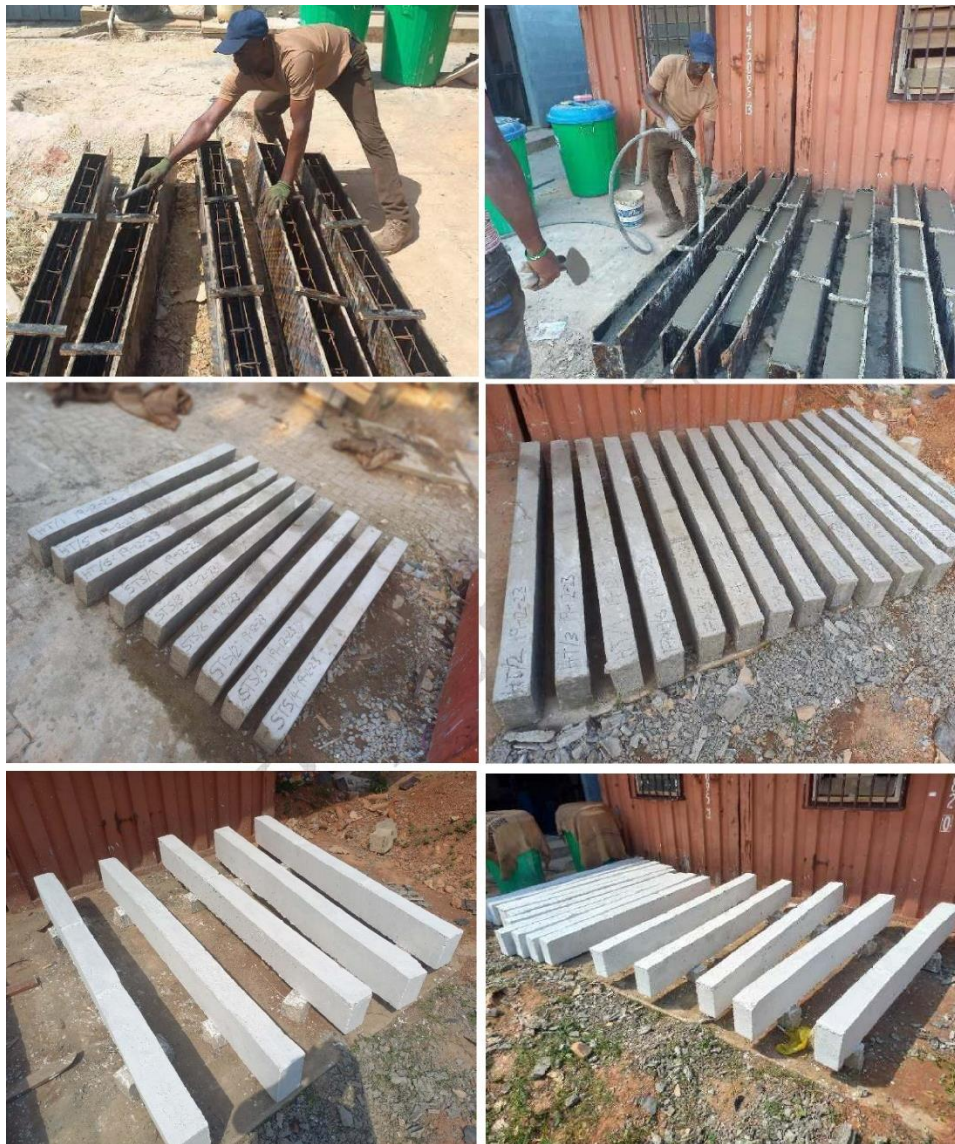
Fig. 2. Preparation of Reinforced Concrete Beam Specimens
