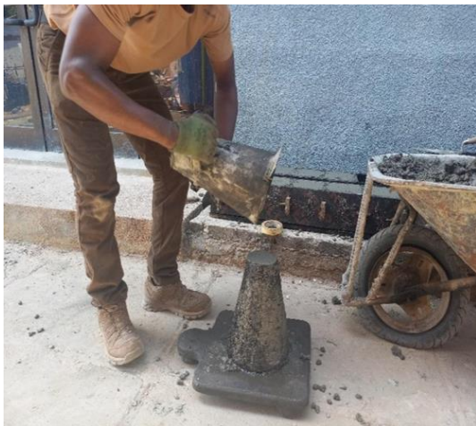
(a) Slump Test on the Fresh Concrete
