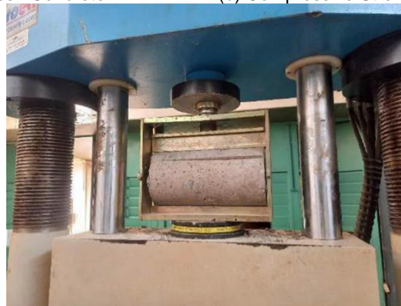
(b) Splitt Tensile Strength Test on Cylinder
