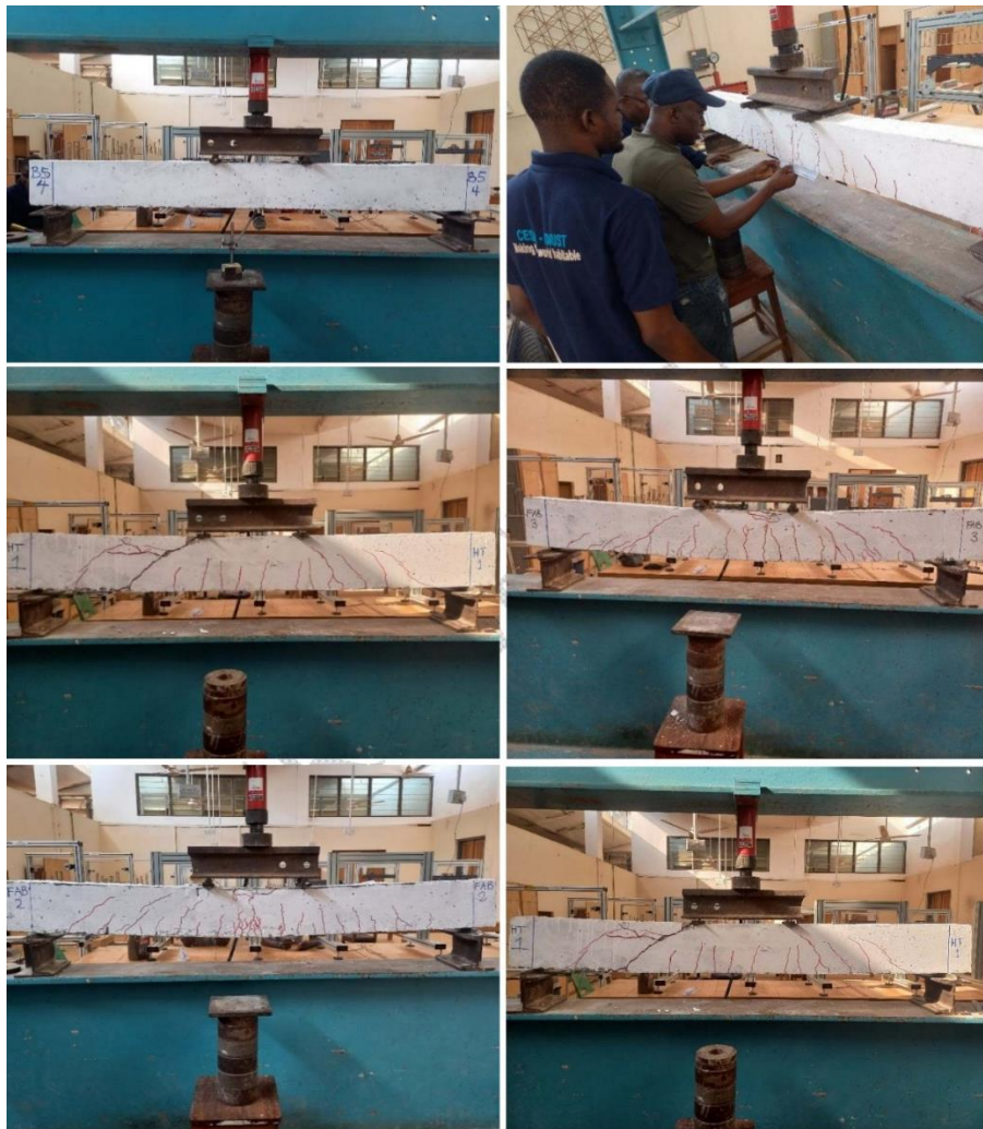
Fig. 3. Beam Specimens during and after Testing
