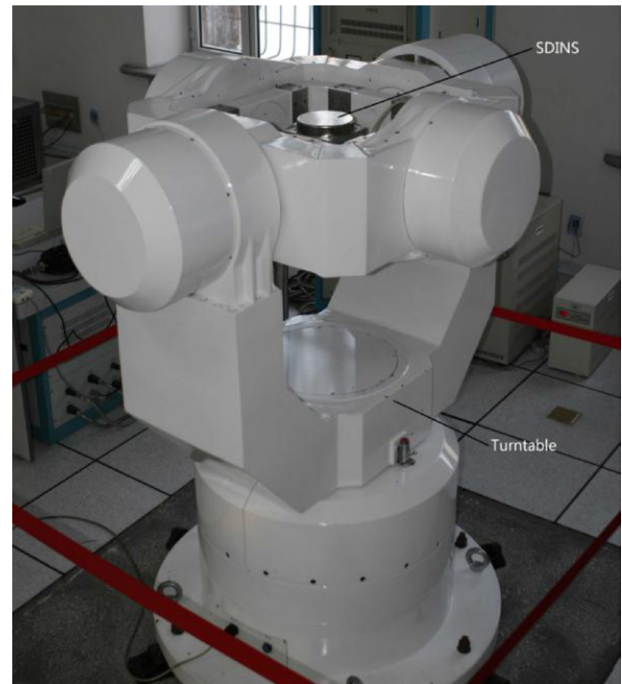
Figure 7. High-precision, three-axis turntable and SDINS.
