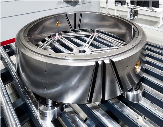
Figure 11. Large gear ring standard with three external and three internal sets of teeth.
