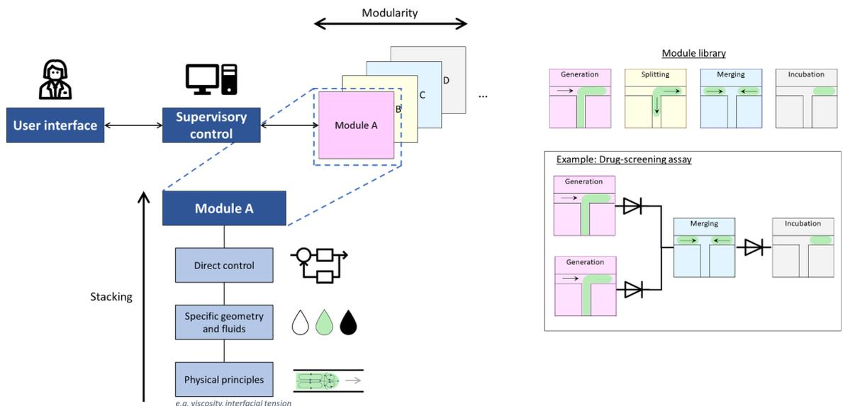
**Figure 1.** Stackable modular platform structure and vision for easy control of individual droplets by end-users. Structure of a stackable modular platform. The vertical direction shows the stacking while the horizontal direction shows modularity. Each manipulation is a module that leverages stacking such that only high-level information from the user is required.
