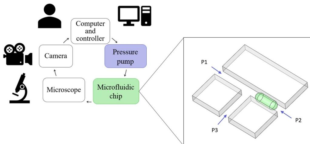
**Figure 7.** Working principle of the combined active and passive platform [211]. The controller calculates the required pressure to apply at each microfluidic chip inlet based on the feedback provided by the microscope, camera, and on-line image processing.
