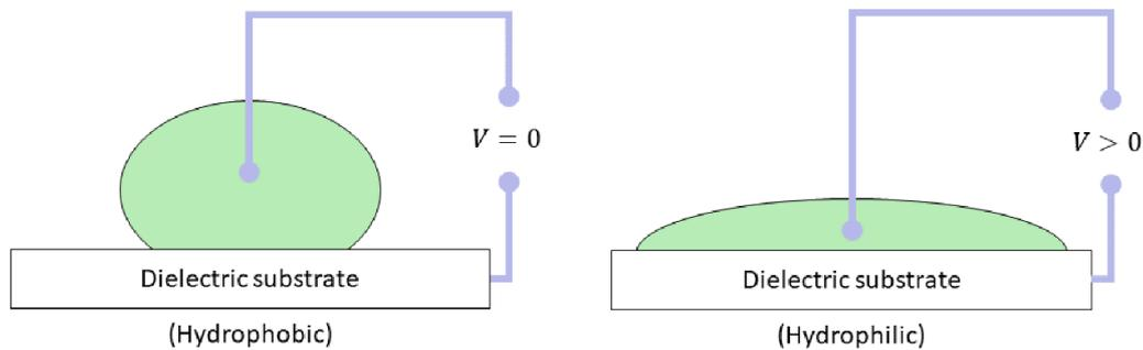
**Figure 3.** Working principle of EWOD platforms [150]. The applied voltage modifies the surface properties from hydrophobic to hydrophilic. The voltage is applied and independently controlled for a grid.
