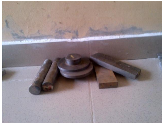
Fig. 12. Slightly machined grey cast iron components
