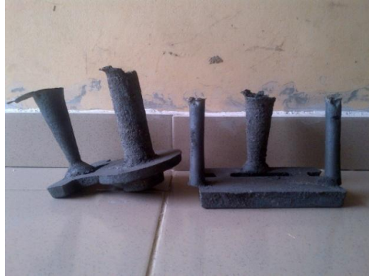
Fig. 11. As-cast components in grey cast iron
