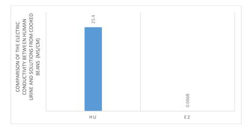
Fig. 6. Electric conductivity of human urine and solutions from cooked beans
