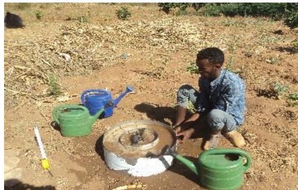
Fig. 3. Measuring infiltration rate using double ring infiltrometer
