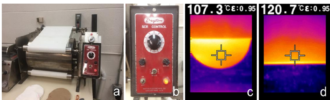
Fig. 1. a) Dayton photo dryer, b) Control unit, c) Handsheet drying, d) Drying felt/cylinder [44]
