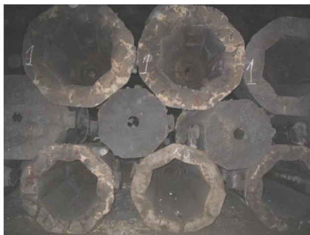
Fig. 7. Deaf-mute molds for forging castings with the weight of 7...10 tons
