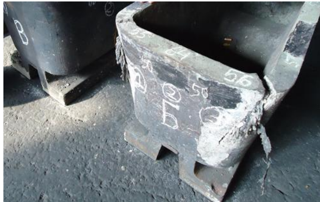
Fig. 1. A broken down mold with leaked alloy traces
