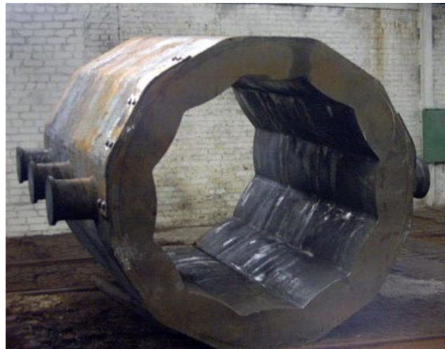
Fig. 8. A through mold for a forging casting (the weight is 42 tons, the wall thickness is 350 mm)
