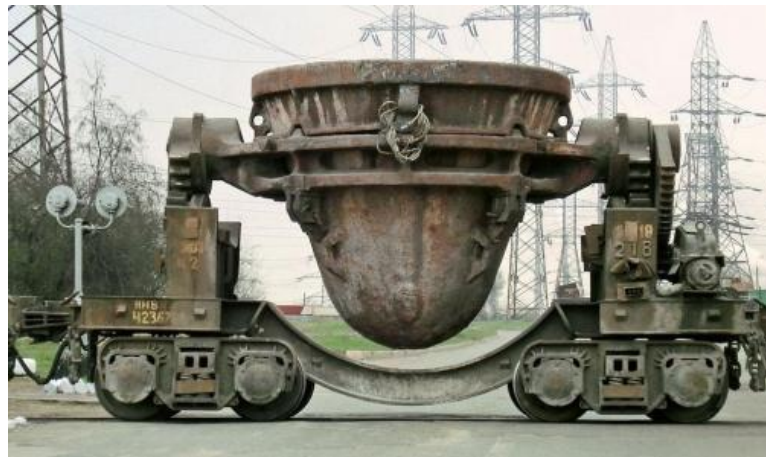
Fig. 9. Slag chalice on a slag-transfer platform (the volume is 15m 3 , the height is 3240 mm, the diameter is 3740 mm)
