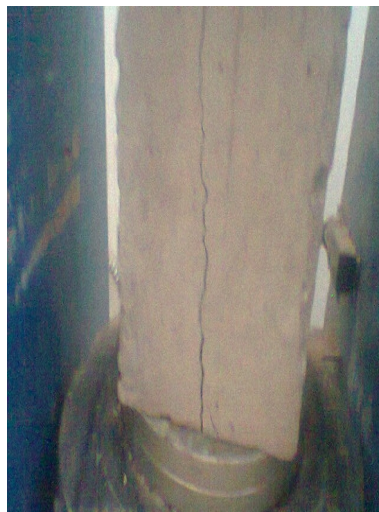
Fig. 4. Failure mode in Bamboo Reinforced Strut
