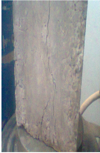
Fig. 5. Failure mode in Steel Reinforced Strut
