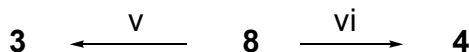
Scheme 3. Reagents and conditions: (v) 8:(H 2 N) 2 C=O – 1:7, 220-230°C (vi) 8:(H 2 N) 2 C=S – 1:3, 200-210°C
